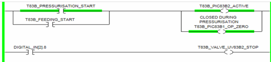
Figure 5. Testing at RUN mode – Tank T-83B
